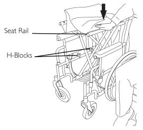
NOTE: DO NOT wrap thumb or fingers under the seat rail. Point fingers and thumb to the inside of the wheelchair.
